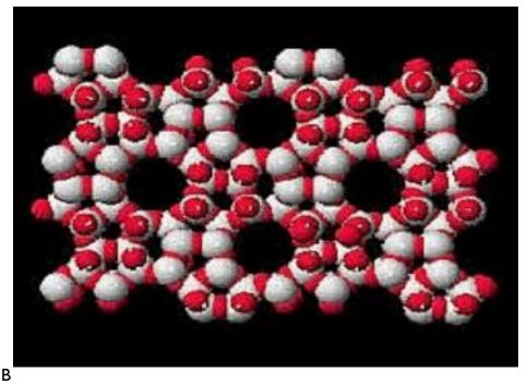
Figure 9: Structures of zeolite, A: framework silicates and B: 3D network of SiO4and AlO4 tetrahedra linked to form channels
