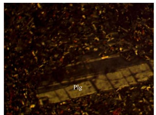
Figure 4: Photomicrograph of basalt showing phenocryst of plagioclase feldspar exhiting both Carlsbad and albite twinning
