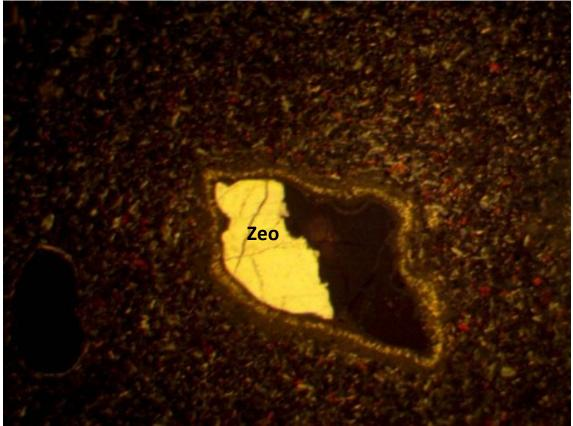
Figure 7: Photomicrograph of zeolite filling empty cavity of basalt
