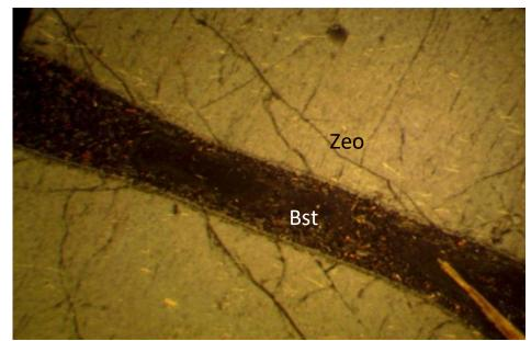
Figure 10: Photomicrograph of basalt showing zeolite being crosscut by groundmass of basalt
