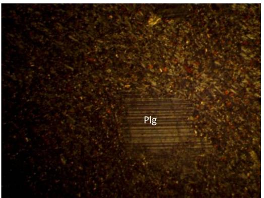
Figure 5: Photomicrograph of basalt showing plagioclase phenocryst in groundmass of olivine, augite, plagioclase and nepheline
