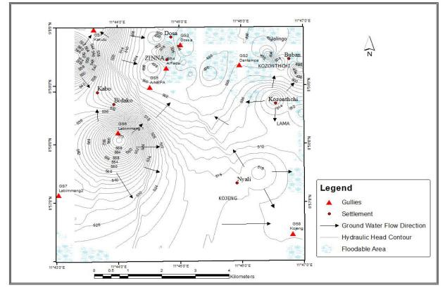
Figure 8: Hydraulic head distribution map showing ground water flow direction.
