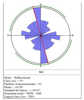
Figure 4: Rose diagram of fractures
