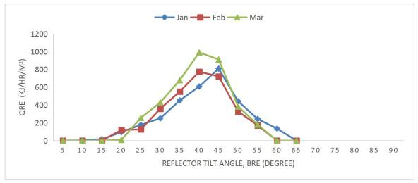
Figure 5: Solar energy absorbed with reflector RE for the first quarter months (January to March) of the year.
