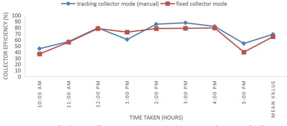
Fig. 8: Variation of collector efficiency (%) with time taken (hours) for drying for fixed and manual tracking modes of the FPC.
