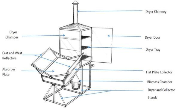
Figure 1: Schematic diagram of the dryer system
