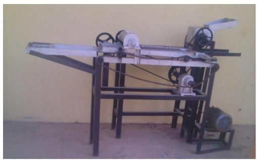
Figure 4. Pictorial View of the Constructed Okra Slicer
