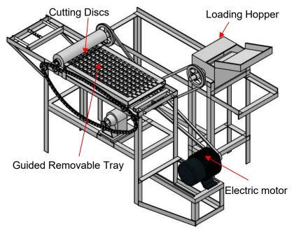
Figure 2. Isometric Projection of the Okra Slicer
