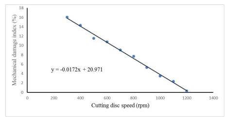
Figure 7. Effect of cutting disc speed on Mechanical damage index of the Okra slicer
