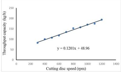
Figure 6. Effect of cutting disc speed on Throughput capacity of the Okra slicer
