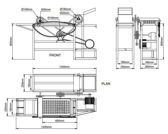
Figure 3. Orthographic Projection of the Okra Slicer
