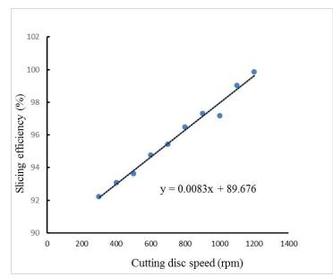
Figure 5. Effect of cutting disc speed on Slicing efficiency of the Okra slicer
