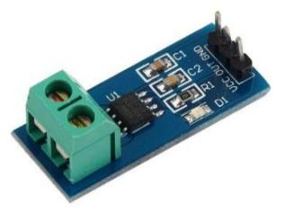
Figure 6: Current sensor module
