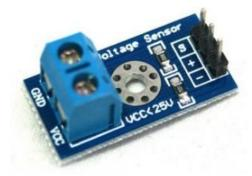
Figure 5: Voltage sensor module
