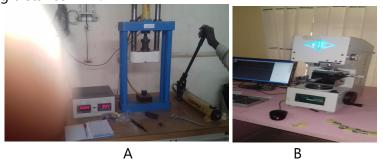
Figure 3: Compression tester (A), Tribometer (B)
