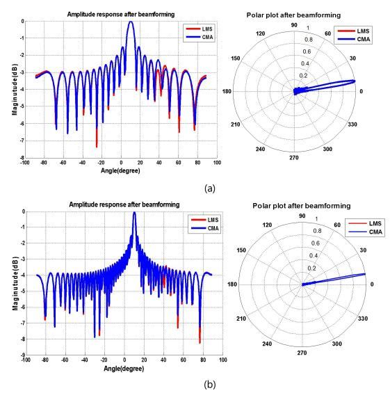
Figure 11: Effect of number of elements N on beam pattern (a) N = 20, (b) N = 50
