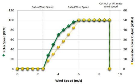
Figure 6: Generator responses to increase in wind and rotor speeds
