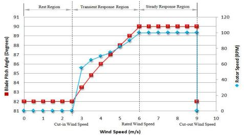
Figure 5: Response of the control mechanism in terms of blade pitch angle and rotor speed
