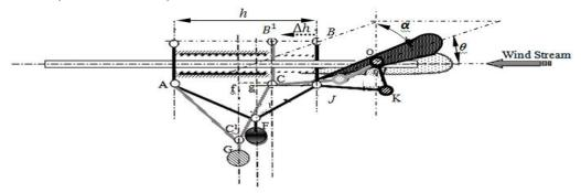
Figure 3: Section of the blade pitch angle control mechanism
