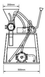
Figure 2: Orthographic Projection of the Hydraulic Press for Sesame Oil
