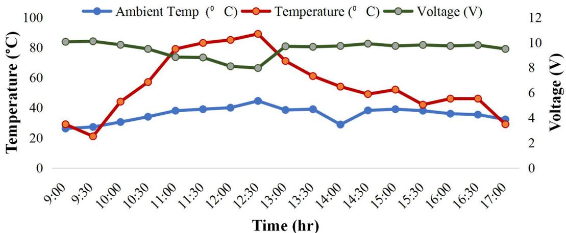
Figure 7: Cooled module temperature and voltage time profile for day three
