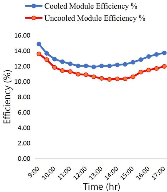
Figure 11: Module efficiency for day 1
