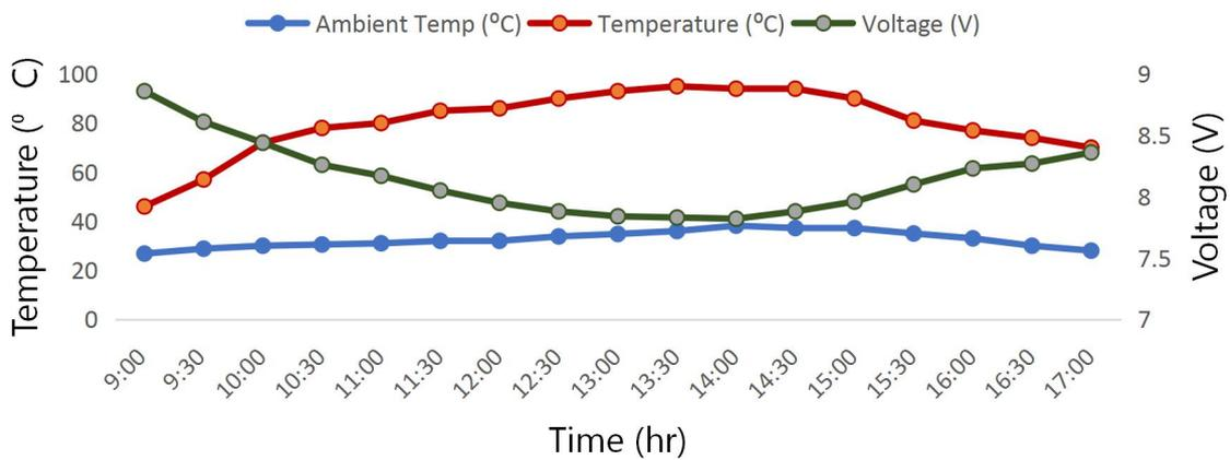
Figure 4: Uncooled module temperature and voltage time profile for day one
