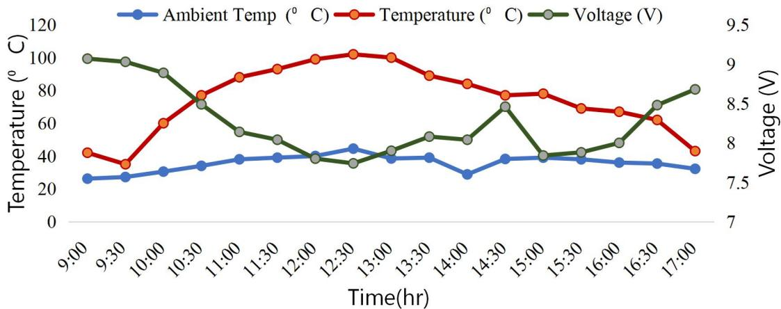
Figure 8: Uncooled module temperature and voltage time profile for day three
