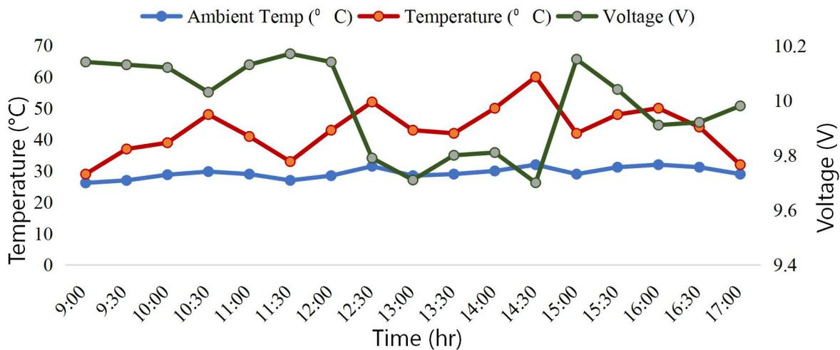
Figure 5: Cooled module temperature and voltage time profile for day two
