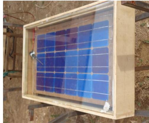
Figure 2: Uncooled module
