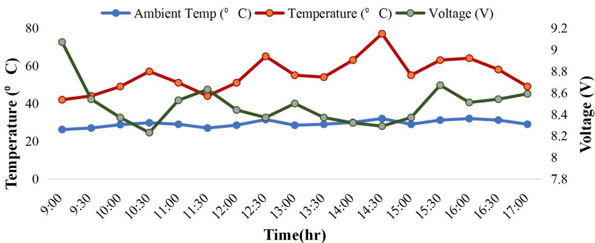
Figure 6: Uncooled module temperature and voltage time profile for day two
