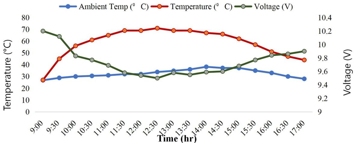
Figure 3: Cooled module temperature and voltage time profile for day one
