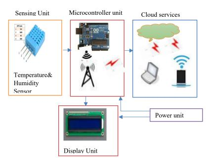
Figure 1 Schematic Diagram of Cloud-Based IoT Monitoring System
