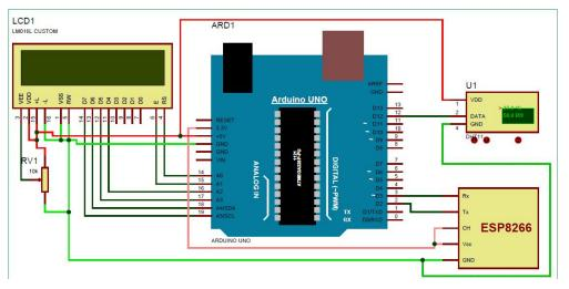
Figure 6 Circuit Diagram of Cloud-based IoT monitoring system
