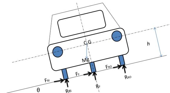
Figure 2: Three-wheeled vehicle on a banked road
