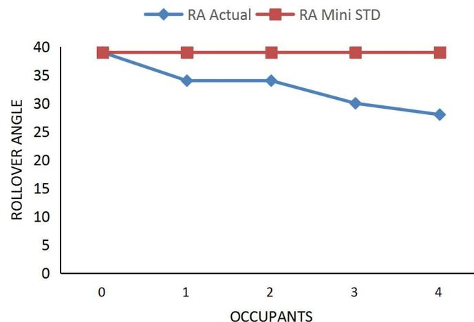
Figure 5: Rollover stability angle versus occupants
