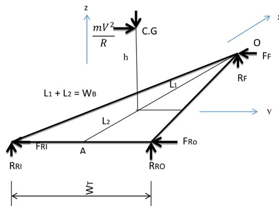
Figure 3: Rollover dynamic stability model
