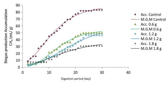
Figure 3: shows the plot of Modified Gopertz.Model Equation for the digesters control,PM CD with 0.6g , 1.2g and 1.8g SP.
