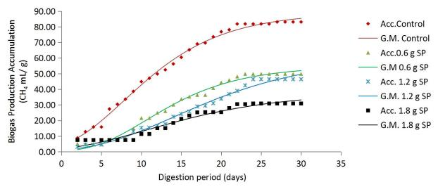
Figure 2: shows the plot of Gompetz Model Equation for control, PM CD with 0.6g, 1.2g and 1.8g SP
