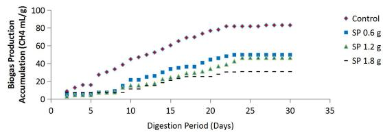
Figure 1: The biogas production accumulation of PM CD 0.6 g SP, 1.2 g SP and 1.8 g SP
