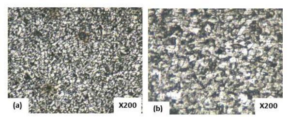
Figure 8: Micrograph of samples at 20% deformation (a) rolled and (b) rolled + stress-relief anneal
