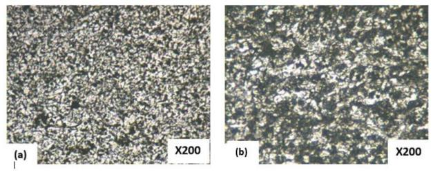
Figure 9: Micrograph of samples at 25% deformation (a) rolled and (b) rolled + stress-relief anneal
