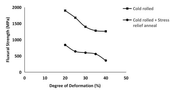
Figure 4: Variation of Flexural Strength with Annealing and Degree of Deformation
