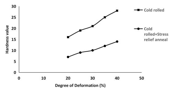
Figure 5: Variation of Hardness with Annealing and Degree of Deformation
