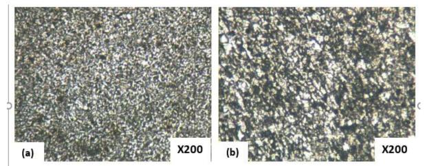
Figure 11: Micrograph of samples at 35% deformation (a) rolled and (b) rolled + stress-relief anneal
