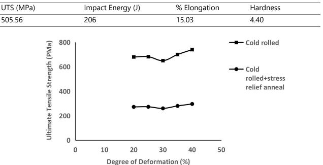
Table 3: Mechanical properties of the As Received Low Carbon Steel.
