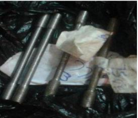
Figure 1: Cylindrical Tensile Test Piece
