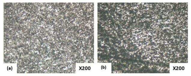
Figure 12: Micrograph of samples at 40% deformation (a) rolled and (b) rolled + stress-relief anneal
