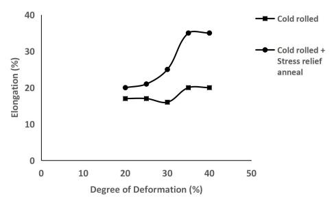
Figure 3: Variation of Elongation with Annealing and Degree of Deformation
