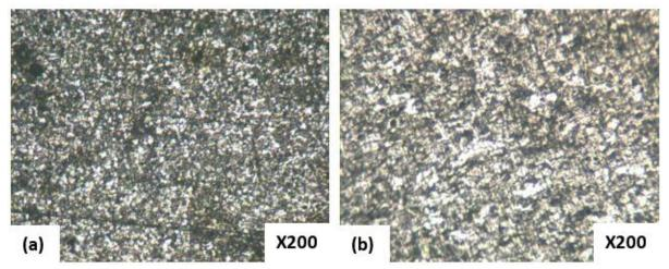
Figure 10: Micrograph of samples at 30% deformation (a) rolled and (b) rolled + stress-relief anneal
