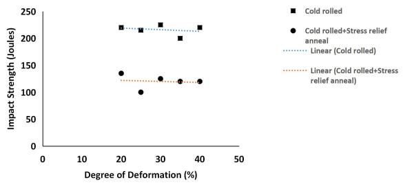
Figure 6: Variation of Impact Strength with Annealing and Degree of Deformation
