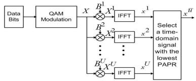
Figure 2: Block Diagram of SLM Technique (Adegbite, et al., 2014).
