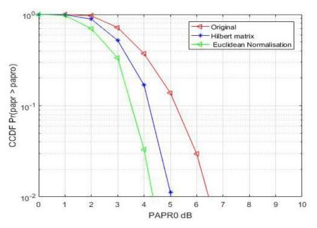
Figure 3: CCDF Plot of PAPR Using Euclidean Normalization.
