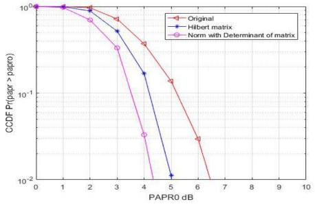
Figure 4: CCDF Plot of PAPR using Normalization with Determinant of Matrix.
