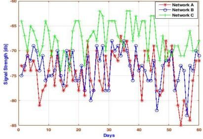
Figure 6: GPRS Signal Strength (dB) against Time (days) for Network A, Network B and Network C in Staff Quarters
