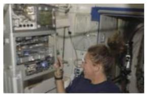
Figure 2: Total Organic Carbon Analyzer Being Used by an Astronaut on the ISS. Image Source: Talbert and Green (2012).
