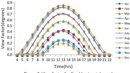
Figure 3: View factor for fixed horizontal panel
