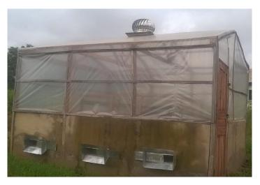
Figure. 2: The NSPRI's Greenhouse Solar Tent Dryer
