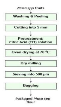
Figure 1: A flow chart showing production of *Musa spp* flours Source: Adeniji *et al.* (2010)
