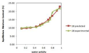
Figure 3: Comparison of experimental and GAB predictive adsorption isotherms of dehydrated African walnut at 28°C
