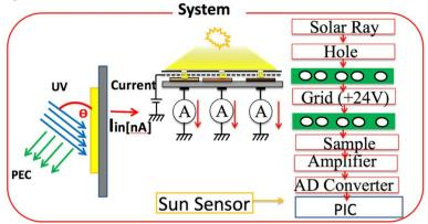
Fig. 3 Schematic of PEC measurement system
