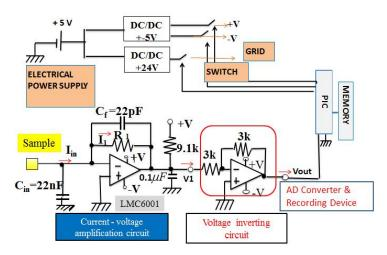
Fig. 2 Schematic circuit of PEC board
