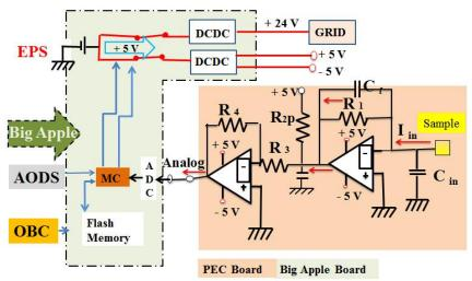
Fig. 5 Schematic diagram of PEC system interfaces (Ewang. 2017)
