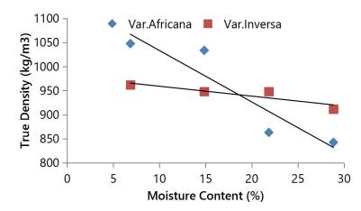
Figure 1: Effect of Moisture Content on True Density of Var. Africana and Var. Inversa
