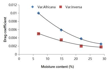
Figure 6: Effect of Moisture Content on Drag Coefficient of Var. Africana and Var. Inversa
