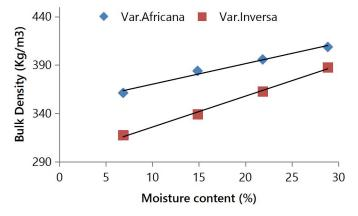
Figure 2: Effect of Moisture Content on Bulk Density of Breadfruit Seed Varieties
