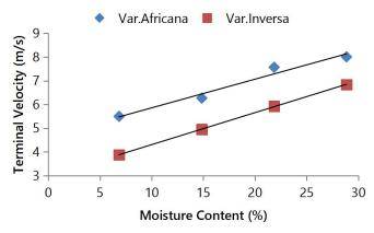
Figure 5: Effect of Moisture Content on Terminal Velocity of Breadfruit Seed Varieties
