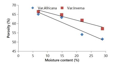
Figure 3: Effect of Moisture Content on Porosity of Breadfruit Seed Varieties
