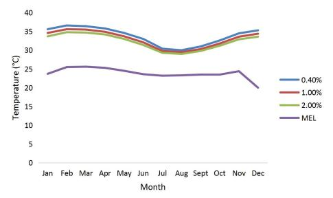
Figure 2: The Mean Coincident Dry-Bulb Temperatures for Ikeja-Lagos from 1995-2009
