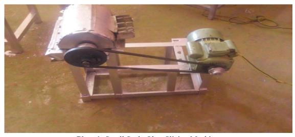
Plate 1: Small Scale Okro Slicing Machine.
