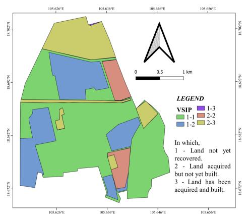
**Figure 5.** Construction area changes in VSIP Nghe An Industrial Park, 2017-2020. (authors' compilation by using Google Earth)
