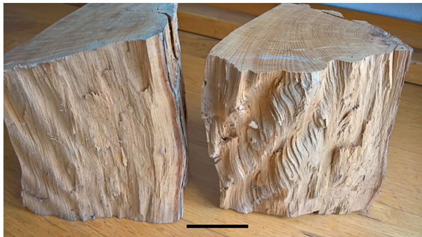
Figure 6 Radial split faces of two beech wood samples with superimposed radial and tangential waviness; in the left sample both periodic patterns moved upward, while, in the right one – in the opposite direction; especially in the right sample superposition of T-wave and R-wave is very clear because of their amplitude – wood grain considered in 3D is inclined not only away and towards the viewer but also away and towards the pith, which in both samples is located on their right side; the apical–basal polarity of both samples is concordant, and their upper transverse surfaces are apical. Scale bar: 70 mm.
