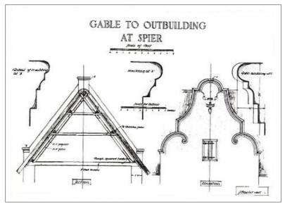
Figure 3: Details of a gable and timber roof structure of Spier outbuilding Source: Pearse, 1968: 19
