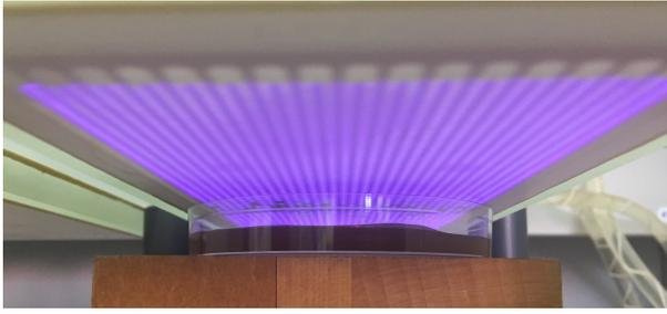
FIGURE 1. Photo of plasma treatment of *Aspergillus brasiliensis* on malt extract agar plates using diffuse coplanar surface barrier discharge (DCSBD) in ambient air.
