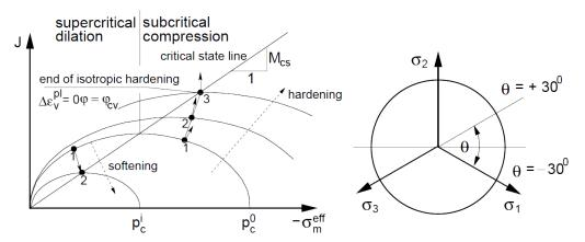
FIGURE 3. Yield surface of the modified Cam-clay model [2].
