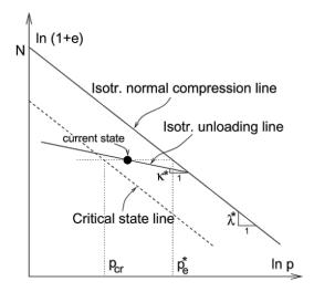
FIGURE 1. Normal consolidation line and swelling line assumed in hypoplastic model for clay [1].
