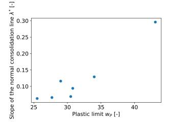
FIGURE 4. Correlation between plastic limit and slope of the NCL assumed in hypoplastic model for clay.
