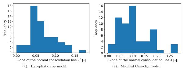
FIGURE 5. Histograms of slopes of the NCL for hypoplastic clay and modified Cam-clay model.
