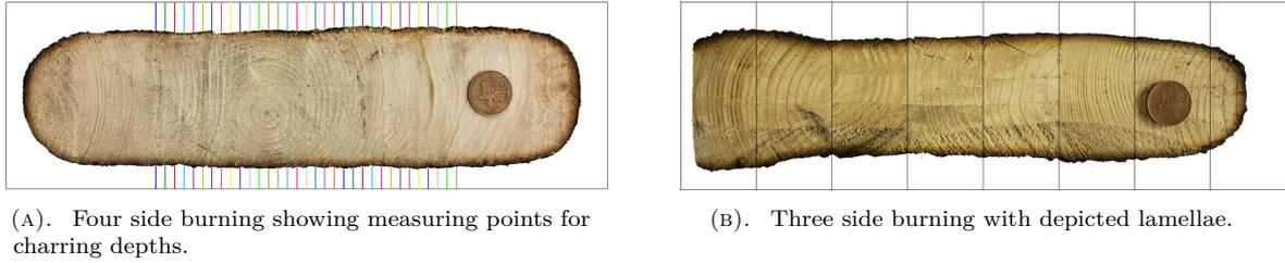
FIGURE 1. Cross-sections with four side burning showing measuring points for charring depths and three side burning with depicted lamellae - both rotated anticlockwise.
