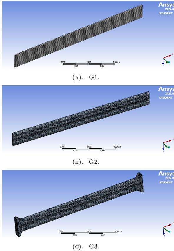
FIGURE 4. Types of beam geometry (Sample 1) with depicted meshes.
