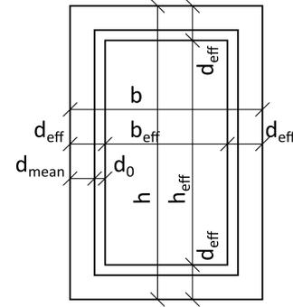
FIGURE 5. Effective cross-section.
