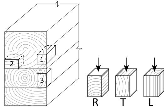
(A). Block cutting scheme. (B). Loading directions.
