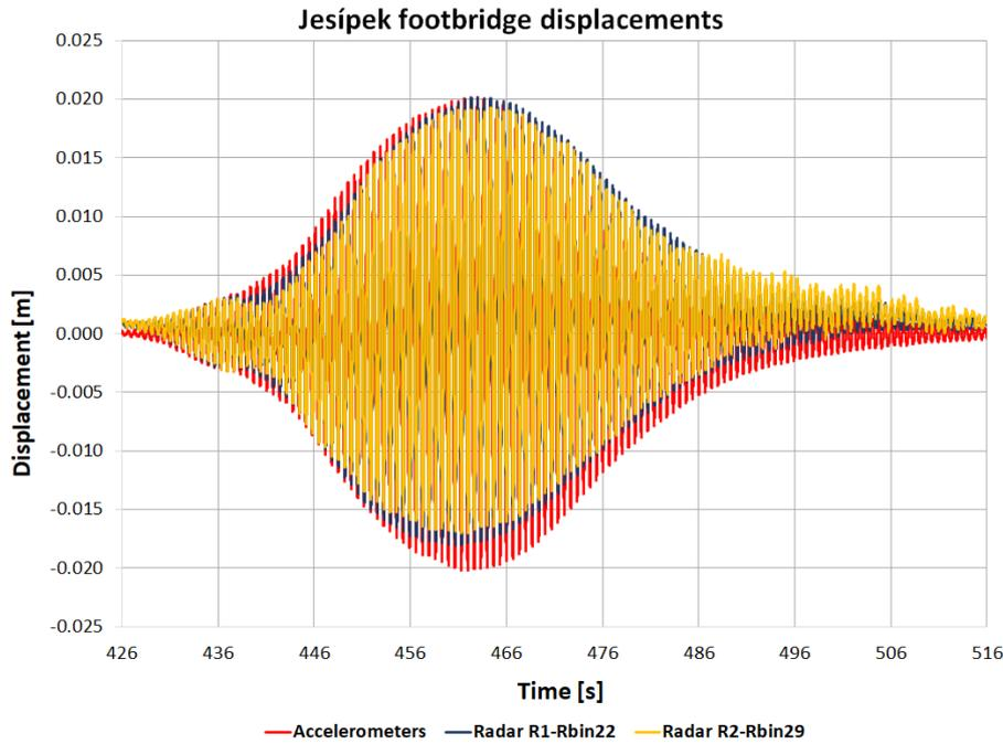
FIGURE 10. Determined displacements in the crossbeam No. 10 position.
