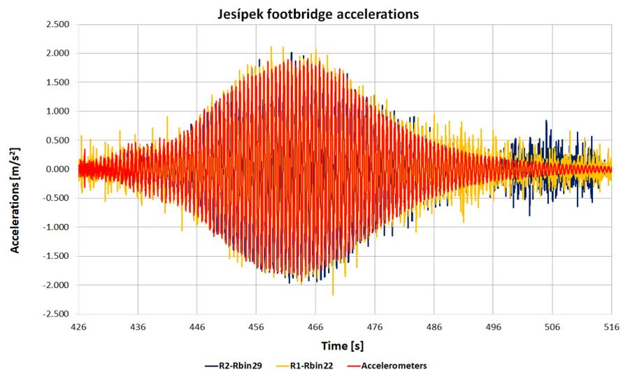
FIGURE 12. Acceleration values in the crossbeam No. 10 position.
