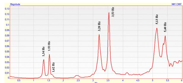
FIGURE 9. The frequency spectrum of acceleration transducer data.
