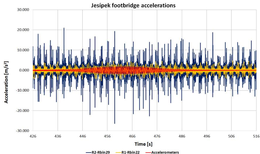
FIGURE 11. Comparison of raw data from radars and sensors.
