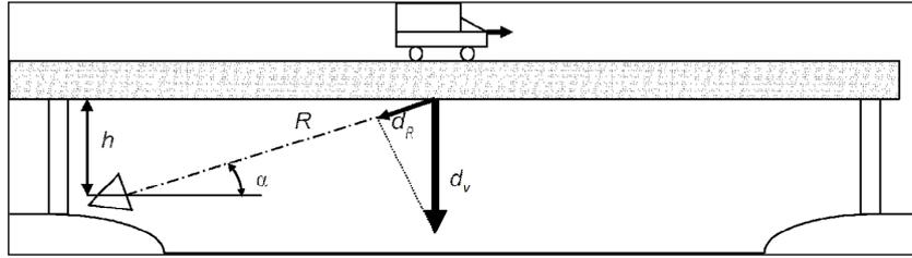
FIGURE 2. Projection of measured deflection to vertical movement [3, 6].
