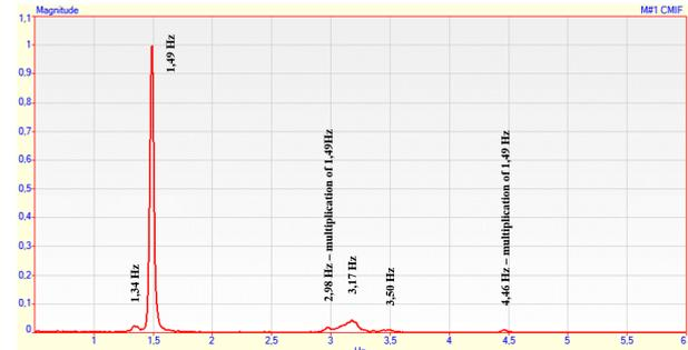
FIGURE 8. The frequency spectrum of radar data.
