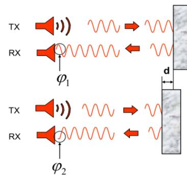
FIGURE 1. Schematic representation of radar interferometry [3].
