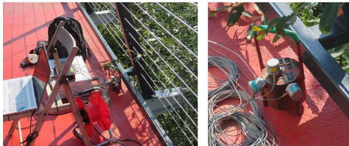
FIGURE 6. Measurement devices prepared in position. A detailed view of the accelerometers.
