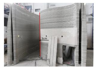
FIGURE 4. Buckling of the 3 meter high wall.
