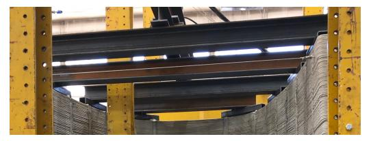
Figure 8. Load distribution system.
