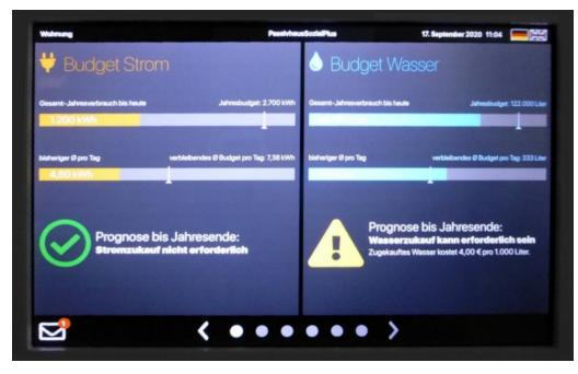
FIGURE 3. Visualisation of the budget for household electricity and drinking water on a display in each apartment.
