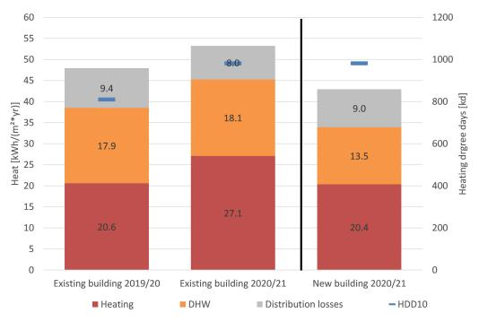
FIGURE 4. Heat consumption for heating, DHW and distribution losses of the refurbished (left and middle column, two heating periods) and the new building (right column, one heating period) as well as heating degree days on site.
