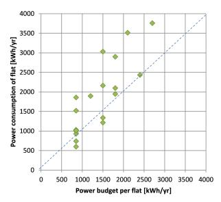
FIGURE 6. Power consumption per flat over power budget per flat for the new building 2020/21.
