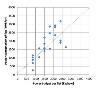
FIGURE 5. Power consumption per flat over power budget per flat for the refurbished building 2020/21.
