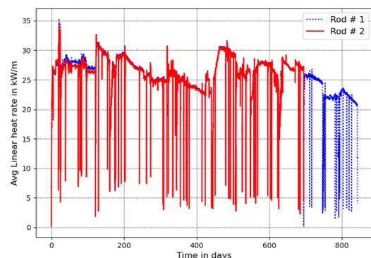
FIGURE 3. IFA 716 average linear heat rate measured during the test.
