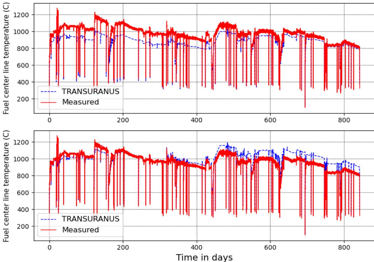
FIGURE 8. Fuel center line temperature measured by thermocouples during the IFA 716 test compared to simulated FCLT using standard thermal conductivity correlation (top) by Hading et al. [12] and high burnup thermal conductivity correlation by Ohira et al. [4].
