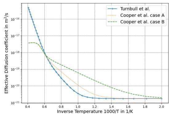
FIGURE 2. Gas diffusivity in undoped  $\text{UO}_2$  fuel using Turnbull et al. model, and gas diffusivity in Cr-doped  $\text{UO}_2$  fuel applying Cooper et al. model.
