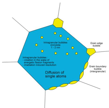
FIGURE 1. Basic mechanisms of fission gas release [2].
