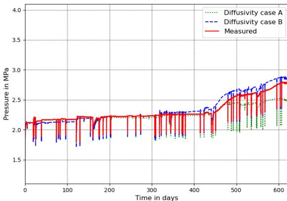
FIGURE 5. Predicted vs. measured rod pressure for rod 1, including the two cases for the diffusivity of doped fuel.
