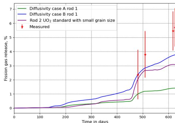
FIGURE 6. Predicted fission gas release for rod 1 and 2.
