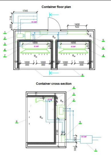
FIGURE 2. Construction scheme of technological equipment of an experimental test cells Twin Rooms. 1 – Cooling source,  $Q_c = 16.4$  kW, MEX EA 117 Z C, 2 – Plate heat exchanger – part of the supply of the cooling source, 3 – Water tank – storage tank Galmet 1401, 4 – Pipe fancoil NXKT3-V1000, 5 – Sill fancoil NXKH3-V600, 6 – Circulating fans – homogeneous thermal field, 7 – Electrical switchgear, 8 – Opening for mounting a new facade sample.
