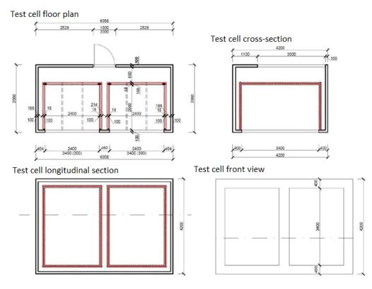
FIGURE 1. Construction schemes of an experimental test cells Twin Rooms for testing advanced facade elements in real conditions of outdoor climate.
