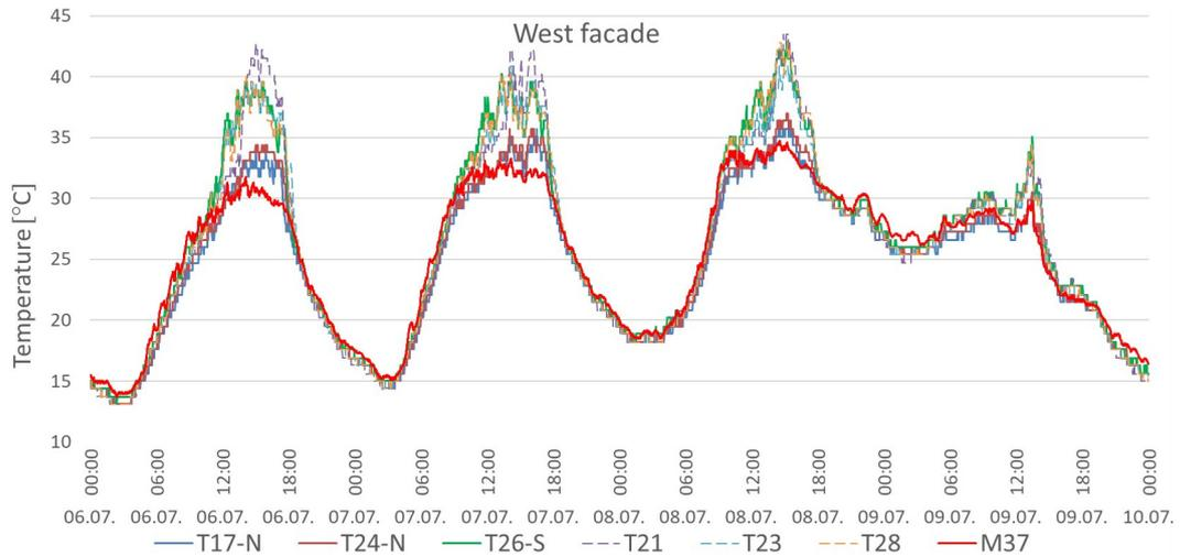
FIGURE 10. Temperature recorded at the FMS sensors on the west facade of the Research Centre building during 6 July 2021 to 9 July 2021.
