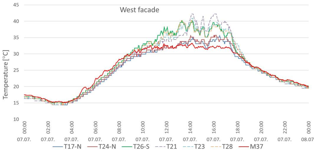
FIGURE 11. Daily temperature course recorded by FMS sensors on the west facade of the Research Centre building during 7 July 2021.
