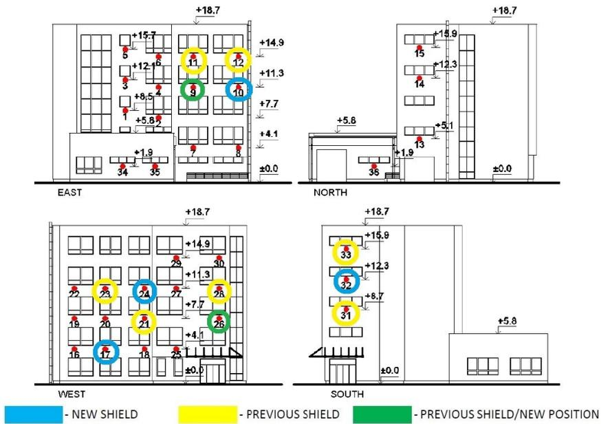
FIGURE 9. Schematic layout of the FMS on the facades of the Research Centre building.
