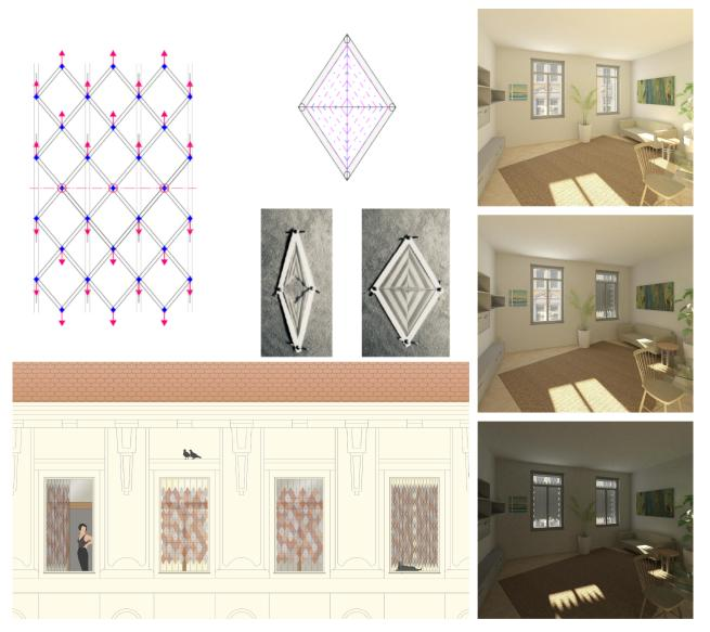
FIGURE 1. Project 1: Rutatus-Blende: Upper left: functional principle, Lower left: Façade view be integration in a Gründerzeit façade, sequence on the right: Shading effect / sun penetration reduction (rendering).
