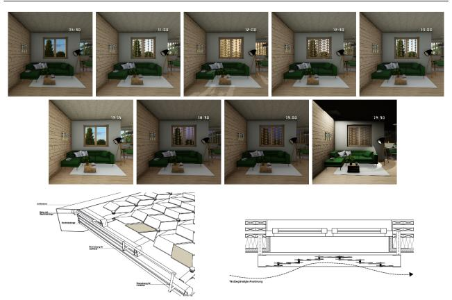
FIGURE 3. Project 3: Sonnensterne: Upper rows: Sequenze of different states of deployment; Lower Row: Isometry and horizontal section of the technical principle of Sonnensterne.
