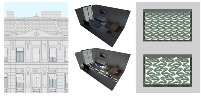
FIGURE 4. Project 4: Fenster-Krausen: Left: Façade view, middle and right, upper row: Fully closed system, middle and right, lower row: Nature-inspired light / radiation transmission.
