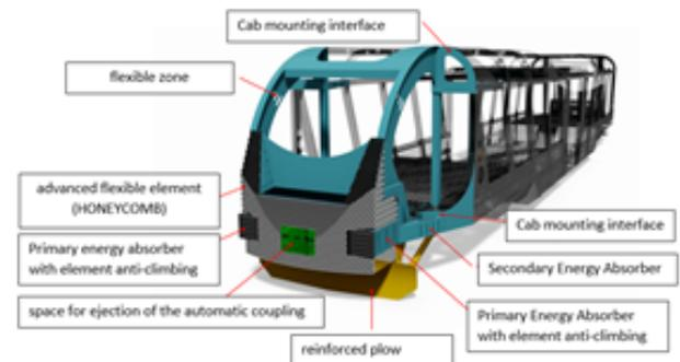
FIGURE 7. Design study of the Rail – electric bus [5].
