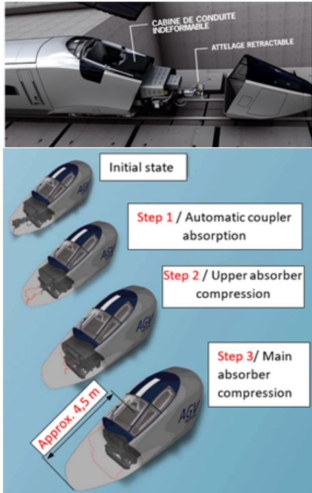
FIGURE 4. Visualization of energy absorption device – HSR train unit AGV [2].
