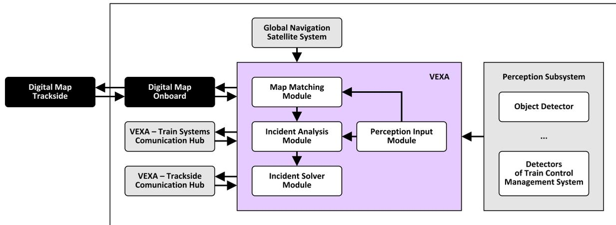
FIGURE 1. Logical architecture of the VEXA system [1]
