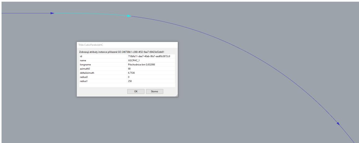
FIGURE 3. Horizontal curves rendered on the basis of the analytical description of the track geometry
