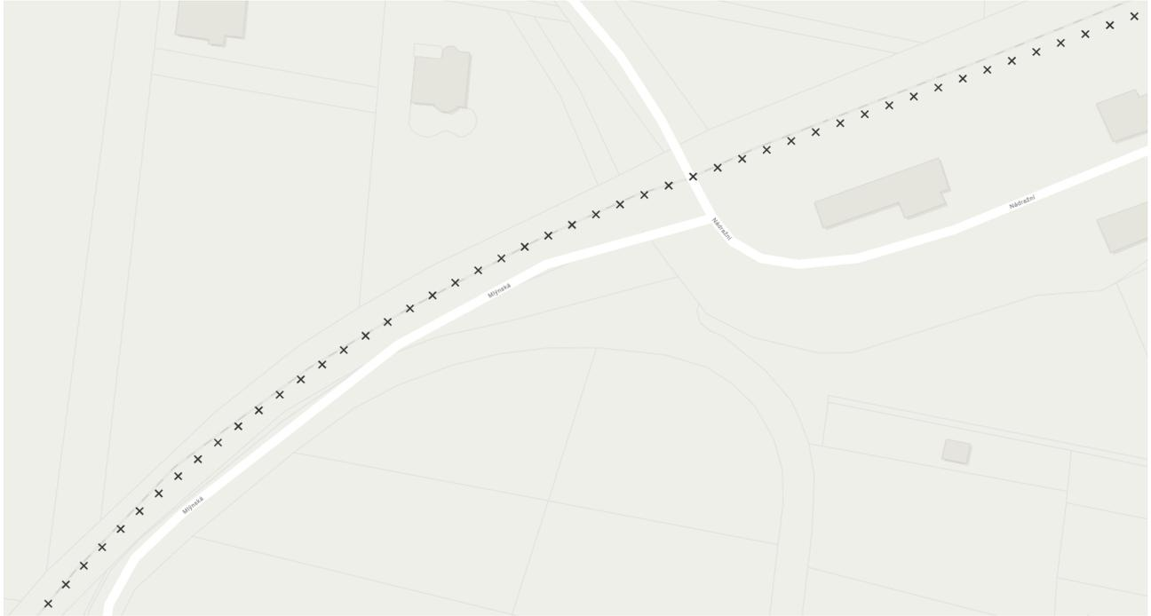
FIGURE 2. Individual points of the track obtained through geodetic survey visualised in the ArcGIS Pro Software
