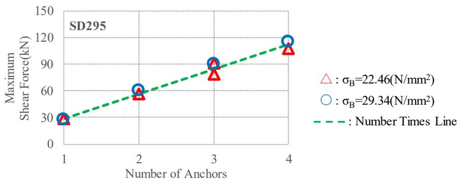
FIGURE 5. Maximum shear force-number of anchors relations. (SD295).
