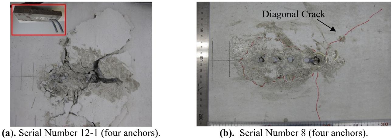
FIGURE 4. Pry-out Failure and Diagonal Cracks (Sign of Pry-out Failure).
