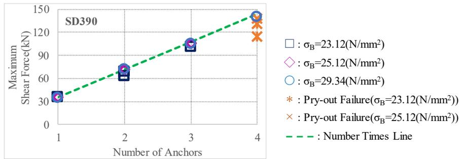
FIGURE 6. Maximum shear force - number of anchors relations. (SD390).
