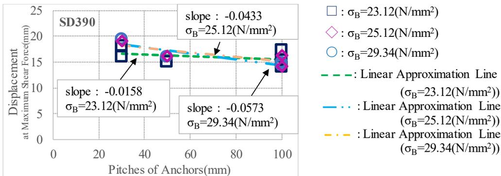
FIGURE 8. Displacement at maximum shear force - pitches of anchors relations. (SD390)
