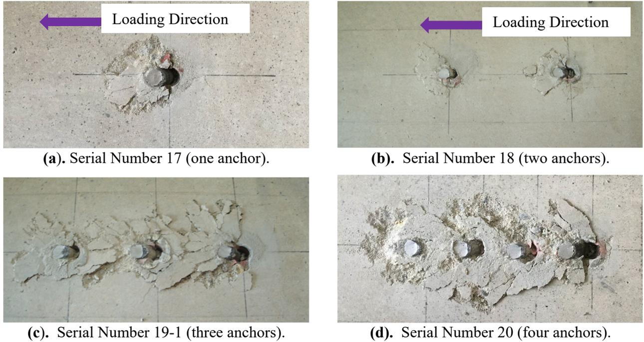
FIGURE 3. Examples for Crack Patterns of Concrete and Shear Ruptures of Anchors.
