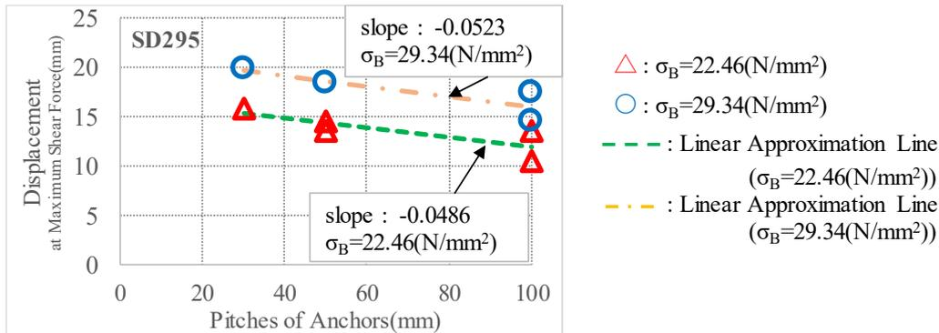
FIGURE 7. Displacement at maximum shear force - pitches of anchors relations. (SD295)
