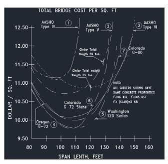
FIGURE 1. Optimum girder spacing cost curves for seven stone concrete girders.
