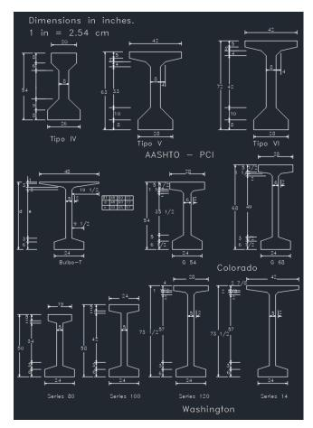
FIGURE 2. Modified girder analyzed (AASHTO, Bulb T, Colorado and Washington).
