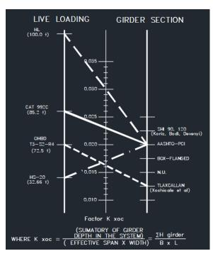
FIGURE 4. Graphic definition of  $K_{xoc}$ , according to live loading and girder type.
