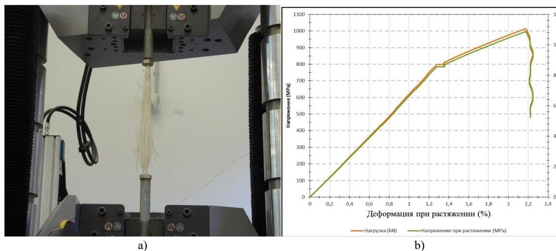
FIGURE 2. FRPR tests. a) The nature of FRPR destruction at the break; b) Tensile stress-strain diagram.
