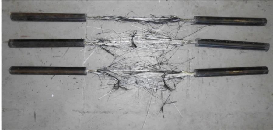
FIGURE 4. ACC-K samples after the rupture test
