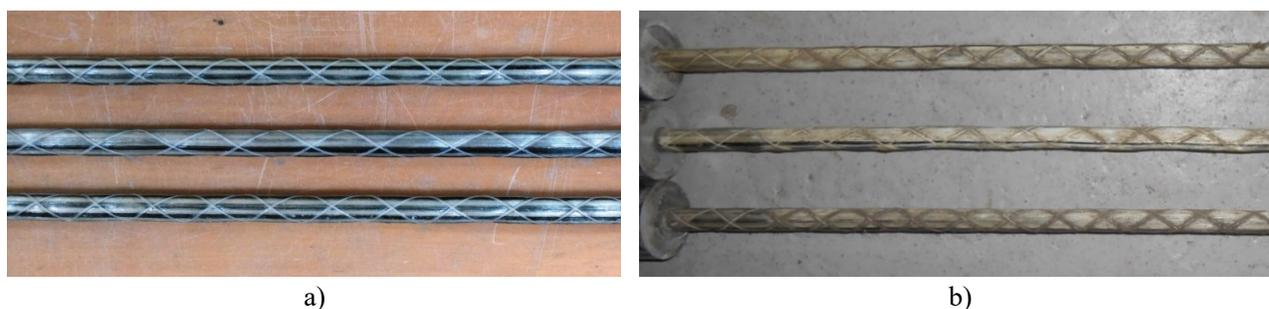
FIGURE 3. Appearance of ACC-K samples before (a) and after (b) exposure in an alkaline medium
