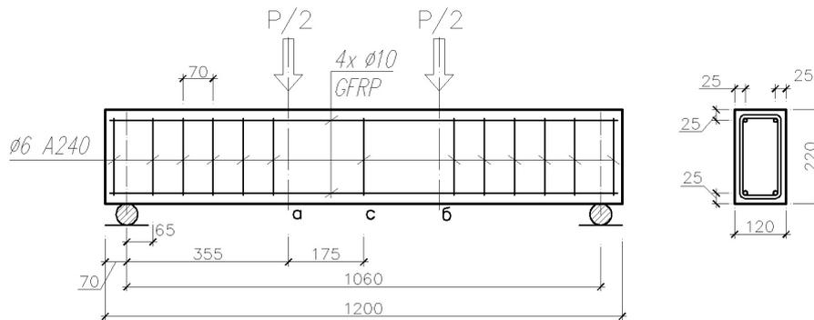
FIGURE 5. Concrete beam reinforcement diagram
