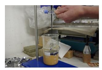
FIGURE 1. An earth sample with methylene blue solution.
