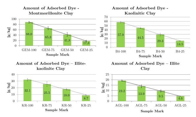
FIGURE 7. Amount of adsorbed methylene blue dye by clay.
