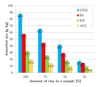
FIGURE 6. Amount of adsorbed methylene blue dye by clays.
