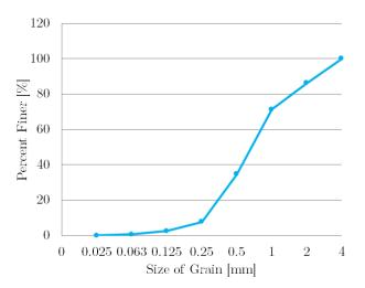
FIGURE 4. Grain curve of sand.
