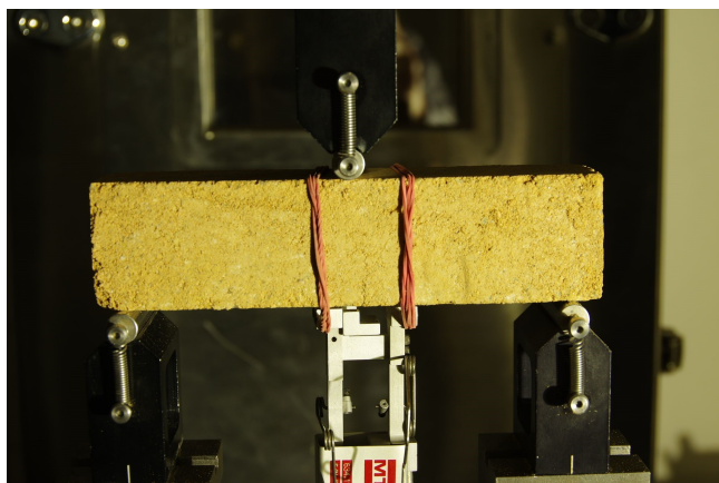
FIGURE 4. The three-point bending test on specimen from rammed earth material.
