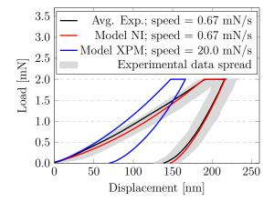
FIGURE 5. Calculated responses of NI and XPM loading with rate dependent viscoplastic model.
