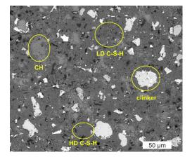
FIGURE 1. Typical SEM-BSE image of cement paste showing individual phases.
