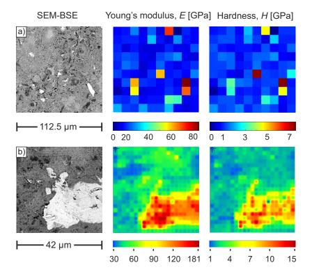
FIGURE 2. SEM-BSE image, Young's modulus, Hardness maps measured by a) NI b) XPM.
