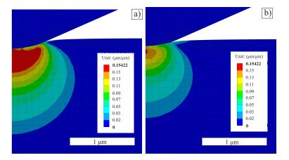
FIGURE 4. Equivalent von Mises strain under the tip at the end of loading a) at time = 3 s, speed = 0.67 mN/s (NI) b) at time = 0.1 s, speed = 20 mN/s (XPM).
