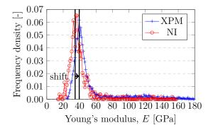
FIGURE 3. Frequency plots of NI and XPM with highlighted shift of the main peak.
