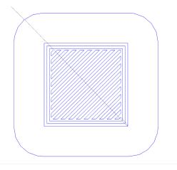
FIGURE 4. G-code visualization of the first layer of a  $20 \times 20 \times 20$  mm cube.
