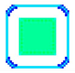
FIGURE 5. Activated voxel elements of a first layer of a  $20 \times 20 \times 20$  mm cube including volume assignment.
