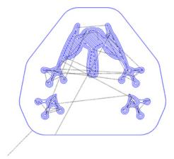
FIGURE 2. Visualization of the movement commands contained in the input file (single layer). Moves with material extrusion are drawn with blue color, moves without extrusion with black color.
