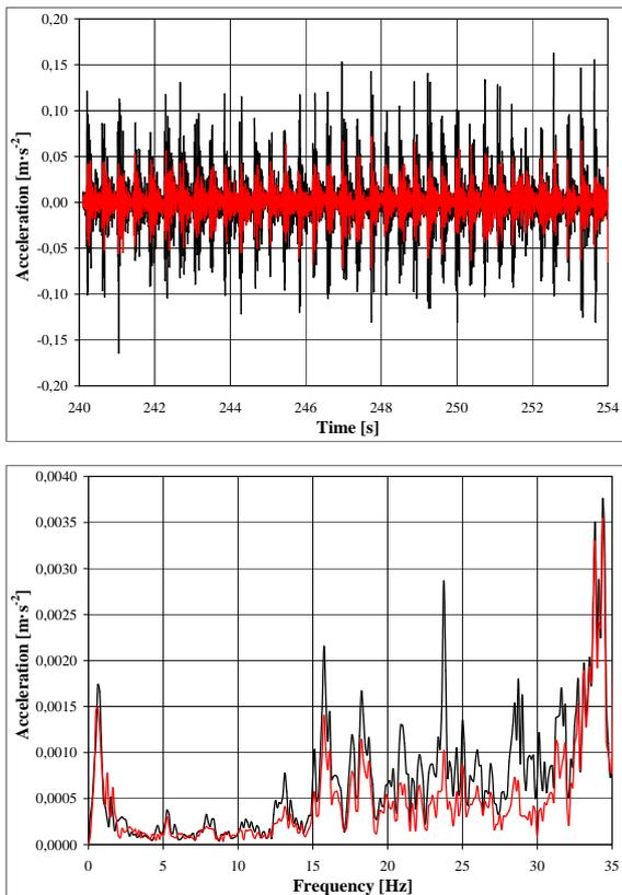
FIGURE 6. Ice-hockey, dynamic response of the stand - Hand-clapping [2].
