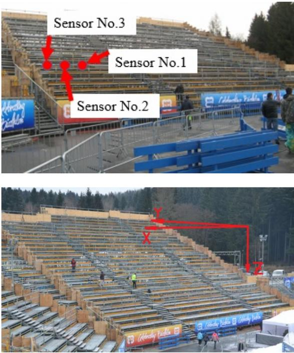
FIGURE 2. Location of sensors at the grandstands and measuring axis sensors [3].
