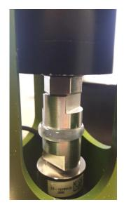
FIGURE 2. Detail of the compressed pure Sylgard 184 sample under 60% deformation in loading chamber
