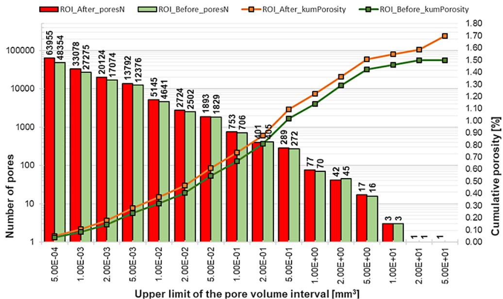
FIGURE 5. Graph of the porosimetric results. Bars in the graph represent histogram of the pore distribution within the investigated ROI before and after the three-point bending fracture test. Curves on the secondary axis represent the cumulative porosity at each pore volume interval.
