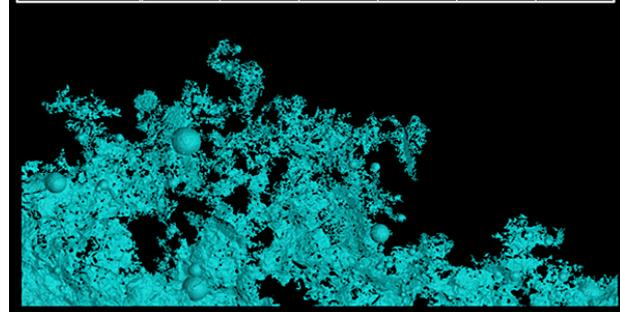
FIGURE 8. Visualization of the extracted fracture surface with the table and graph of the values obtained using box counting algorithm.
