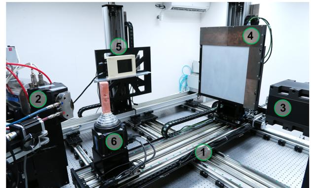
FIGURE 2. TORATOM tomography system: Active damped anti-vibration table with high-precision CNC positioning system (1) holds two imaging pairs of the X-ray tube (2, 3) and detector (4, 5) in an orthogonal arrangement with shared rotary stage (6) accommodating the investigated specimen.
