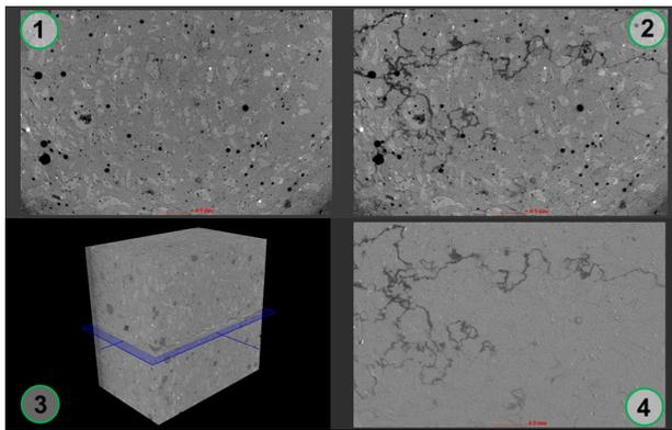
FIGURE 6. Visualization of tomographic cross-sections taken in the same place parallel to the direction of the crack propagation ( $xy$  plane). 1) Visualization of the cross-section before three-point bending; 2) Visualization of the cross-section after three point bending; 3) Plane representing the position of the visualized cross-sections (orientation of the volume corresponds to Figure 3); 4) Differential image with highlighted differences (cracks).
