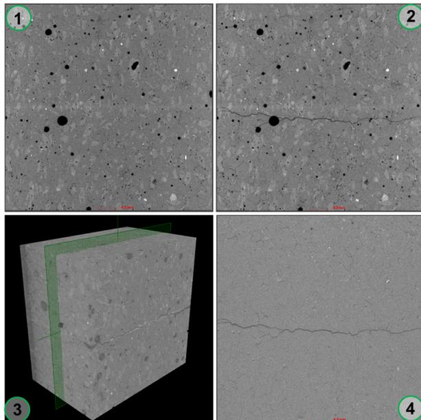
FIGURE 7. Visualization of tomographic cross-sections taken in the same place perpendicular to the direction of the crack propagation ( $xz$  plane). 1) Visualization of the cross-section before three-point bending; 2) Visualization of the cross-section after three point bending; 3) Plane representing the position of the visualized cross-sections (orientation of the volume corresponds to Figure 3); 4) Differential image with highlighted differences (cracks).
