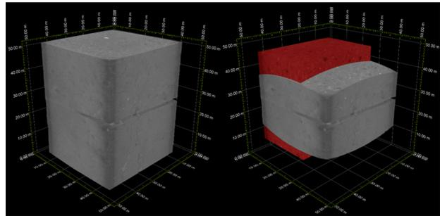
FIGURE 3. Visualization of the obtained 3D model of the scanned area. Part indicated by the red color specifies the volume used for the determination of porosimetric parameters and further investigation of the crack spatial distribution.
