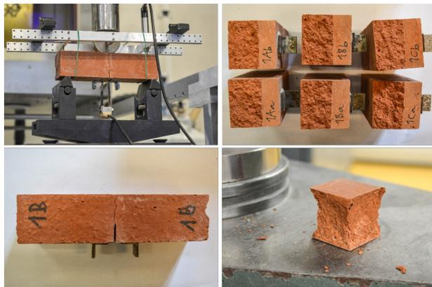
FIGURE 1. Illustration of fracture test in three-point bending (left), selected specimens after the fracture tests in three-point bending (top right), and specimen after test in compression (bottom right).
